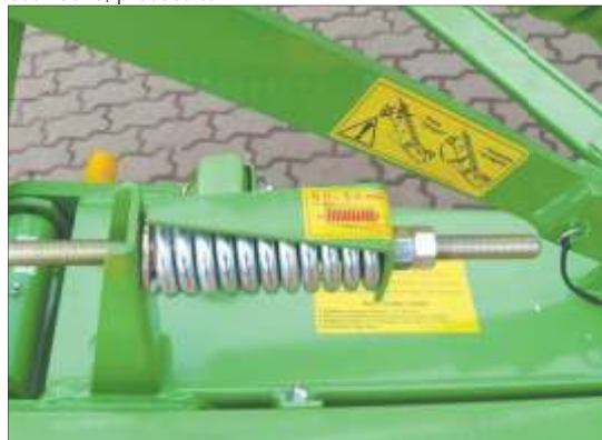
When tightening V-belts check if the distance between plate tip and holder is 5 mm.
