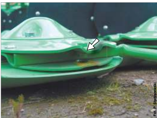
Not only do the knives wear. During usage knife holder's pin wears as well.
