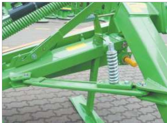
If the safety device breaks away too easily, tighten up the spring approximately 1-2 mm.
