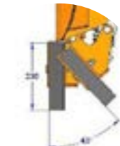
Trip back mechanism, allows for clearing bar deflection up to 43° and the section to trip back and over, which therefore allows to slide over 24 cm (9 1/2 „) high obstructions.
