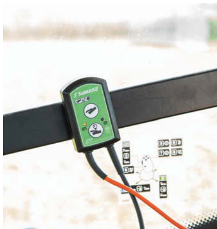
Lifting the mower in and out of work is done via this neat little in-cab controller.
