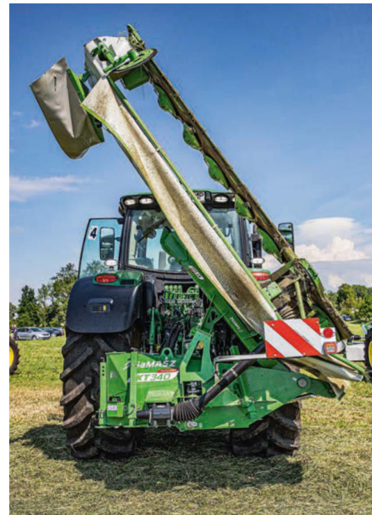
Folding over centre to 125° helps to keep the 3.40m mower balanced on the tractor's linkage as well as reducing overall height.
